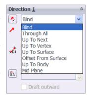
Scroll down to and select **Mid Plane**. Set **D1** to a size larger than the diameter of the semi-circle. **125mm** works well. Choose OK to confirm the changes.
