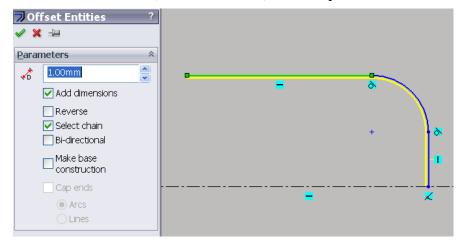
Join the end points of offset entities using the 'Line' command as shown
